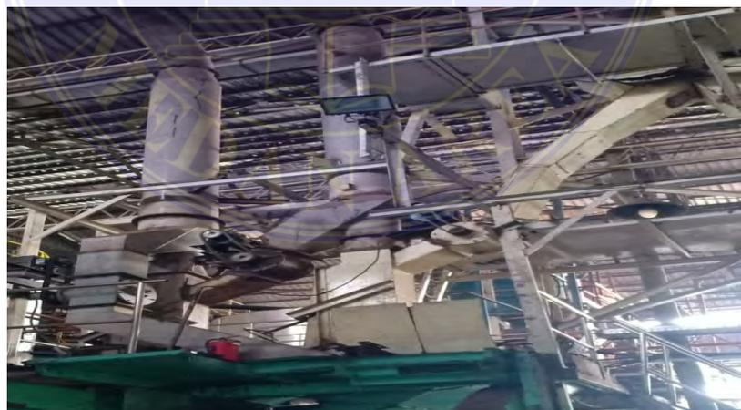
Gambar 3.42. *Light Tenera Dusting Separator*
