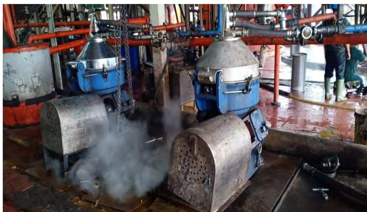
Gambar 3.29. *Sludge separator*
