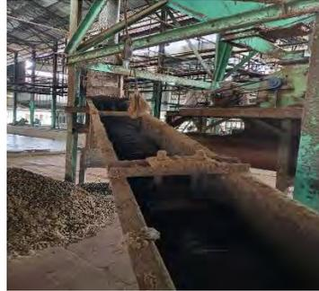
**Gambar 3. 30** *Inclide distribusi bunch conveyor*
