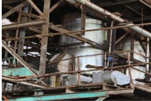
**Gambar 3. 38** *Continuous settling tank*
