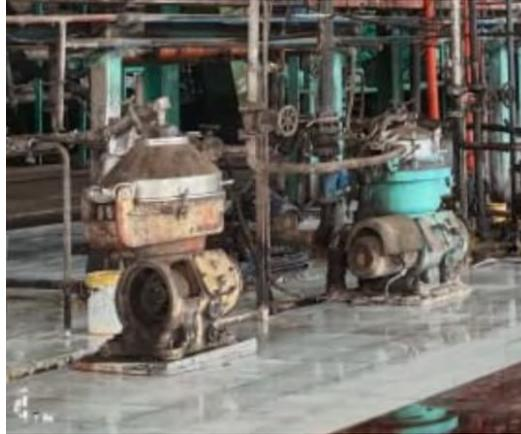
**Gambar 3. 40 *Sludge separator***
