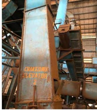
**Gambar 3. 48** *Cracked mixture elevator*
