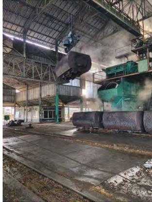
**Gambar 3. 26 *Hoisting Crane***
