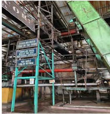
**Gambar 3. 28 *Inclined fruit bunch conveyor***
