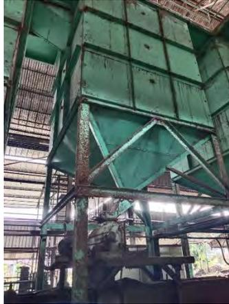
**Gambar 3. 19** *Ripple mill*
