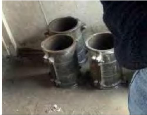
Gambar 3.27 Bekisting Silinder Sample
