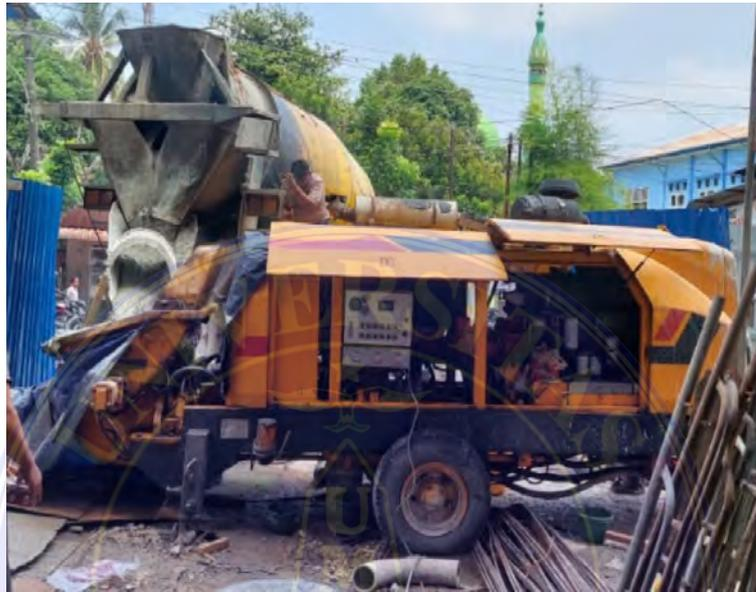
Gambar 3.11 Pompa Beton/*Concrete Pump Truck*
