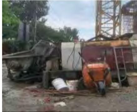
Gambar 3.11 *Concrete Pump*
