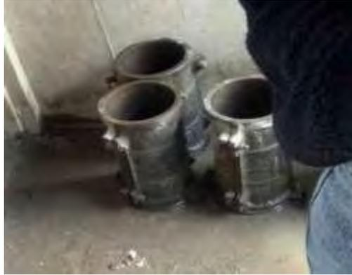
Gambar 3.27 Bekisting Silinder Sample
