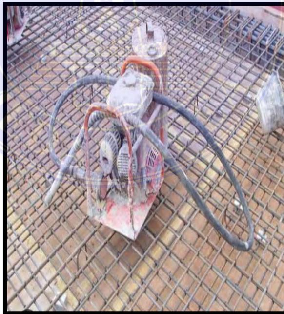
*Gambar 3.1 1 Beton Vibrator*
