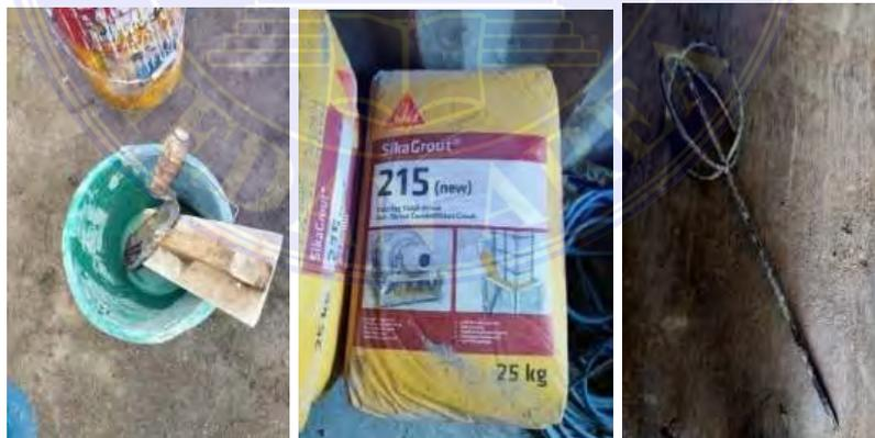
Gambar 3.1.26 Peralatan Grouting
