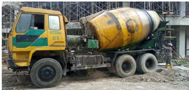
Gambar 3.1 *Ready Mixed Concrete Truck*
