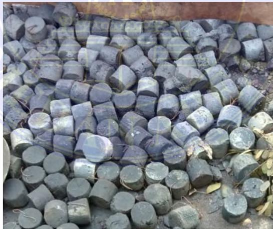
Gambar 3.13 *Beton Decking*
