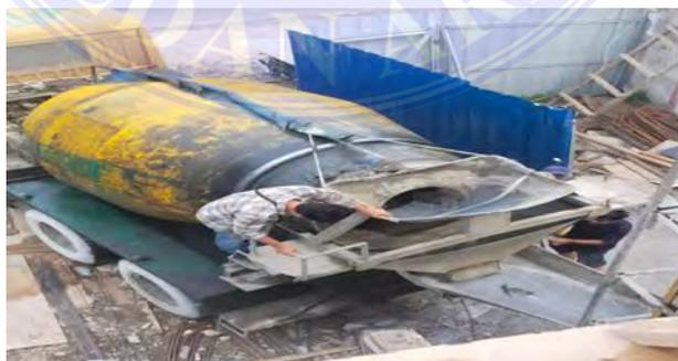
Gambar 3.8 *Truck Mixer Beton*
