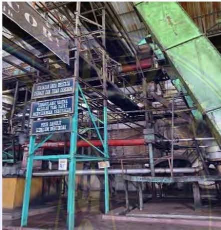
**Gambar 3. 28 *Inclined Fruit Bunch Conveyor***
