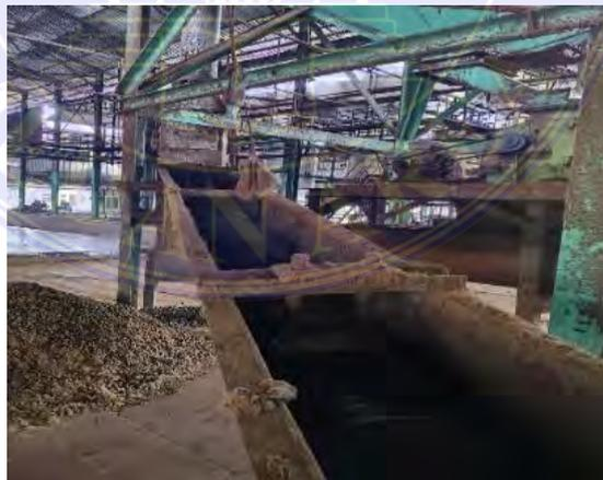
**Gambar 3. 30 Inclide Distribusi Bunch Conveyor**
