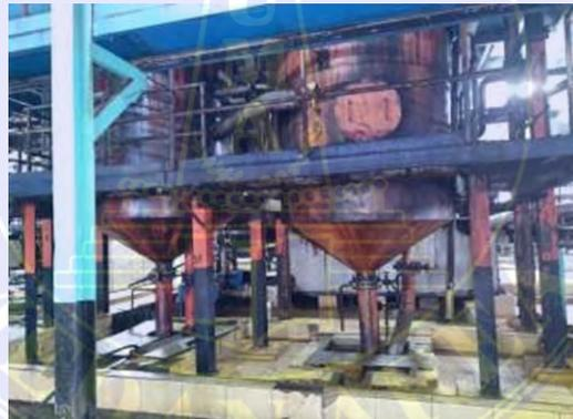
**Gambar 3.21 Sand Trap Tank**
