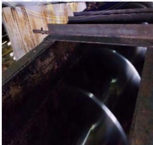
**Gambar 3. 14** *Under Thresher Conveyor*
