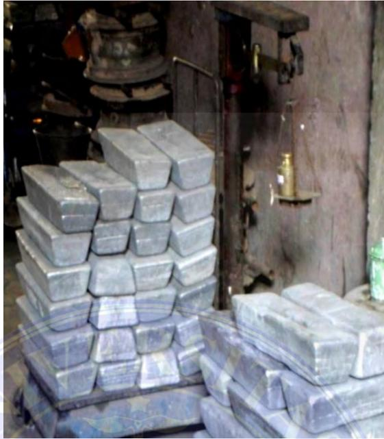
**Gambar 3.1** Bahan baku aluminium (ingot)
