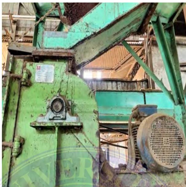
**Gambar 3. 17. Ripple Mill**
