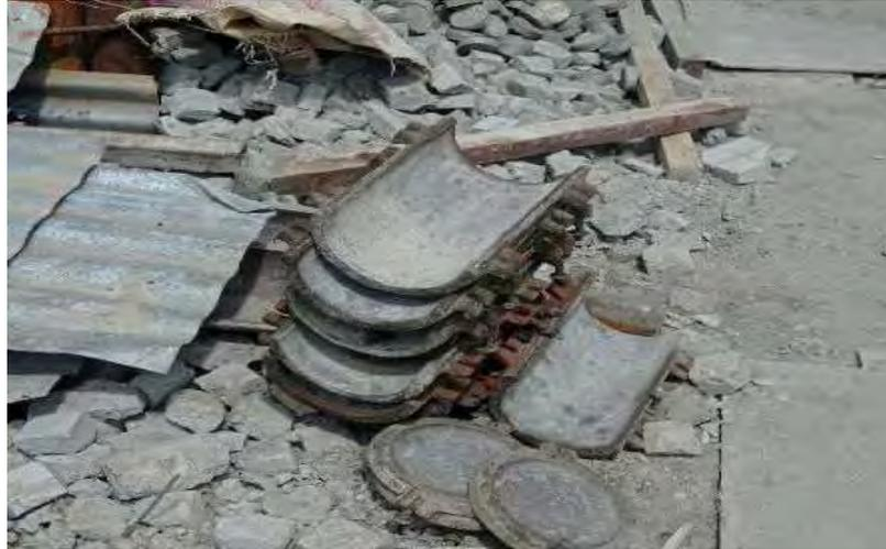
Gambar 3.24 Bekisting Slinder Sampel
