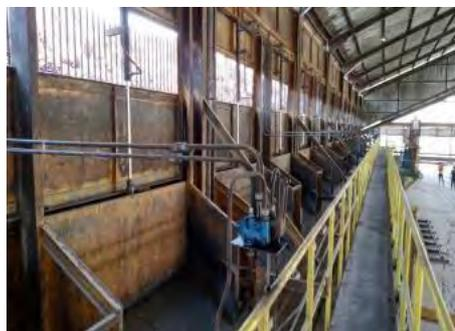
**Gambar 3.12 *Vibro Separator/ Vibrating Screen***
