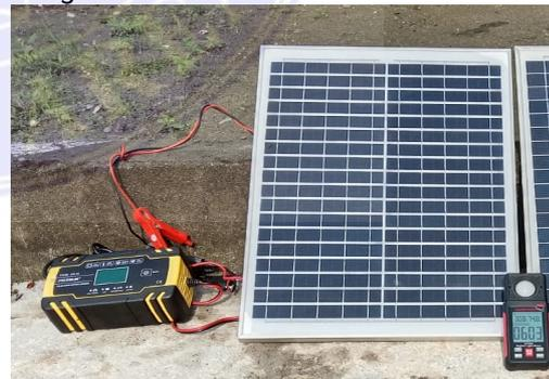
Gambar 2: Instalasi Pengukuran Panel Surya Polycrystalline
