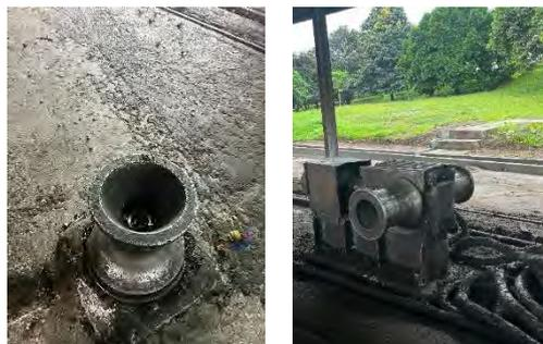
**Gambar 3. 5 Capstand & bollard**
