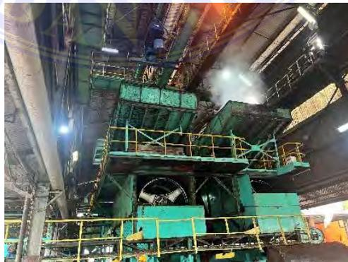
**Gambar 3. 8 Tromol Pembanting (*Thresher*)**
