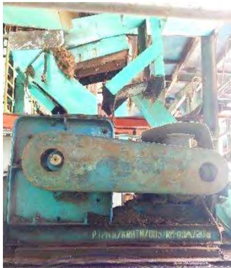
Gambar 3. 40 Ripple Mill
