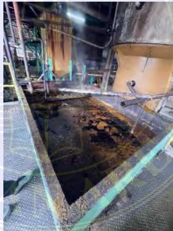
**Gambar 3. 13 Tangki Minyak Kasar (*Crude Oil Tank*)**
