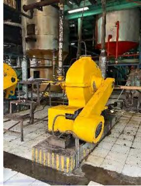
**Gambar 3. 16 Sentrifuse Minyak (*Oil Purifier*)**
