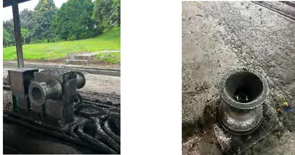
**Gambar 3.5** *Capstand & bollard*
