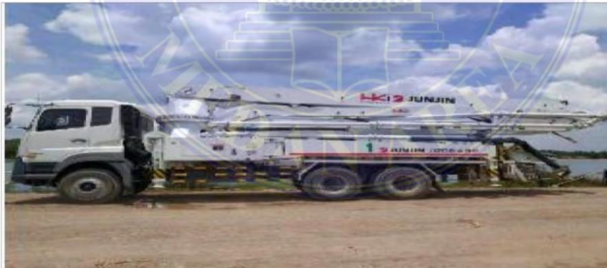
Gambar 10 *Concrete pump*
