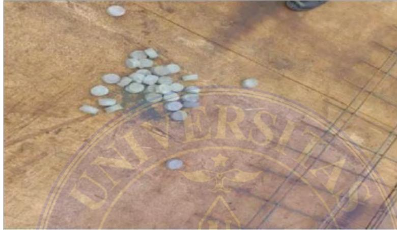
Gambar 22 *Beton Decking*
