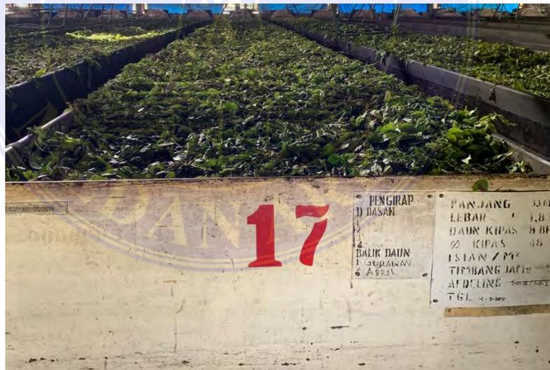
Gambar 3.15 *Withering Trough* (WT)
