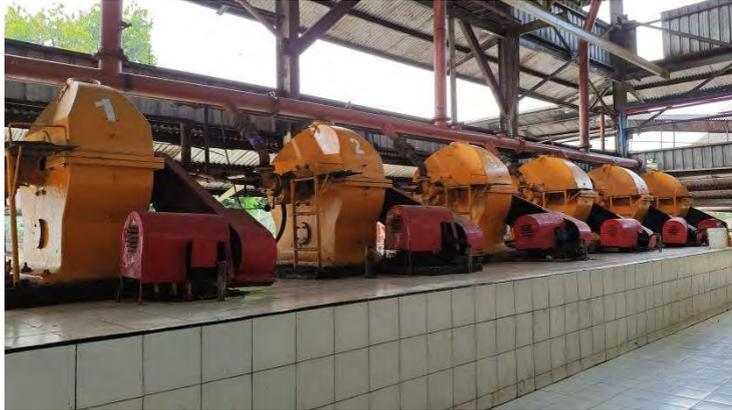
**Gambar 3.38 Sludge Centrifuge**
