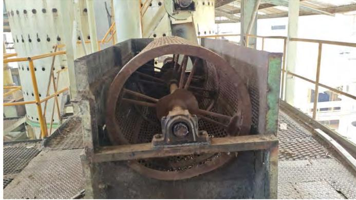
**Gambar 3.47 Nut Grading Drum**
