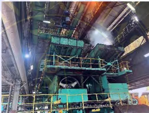
**Gambar 3. 8 Tromol Pembanting (*Thresher*)**
