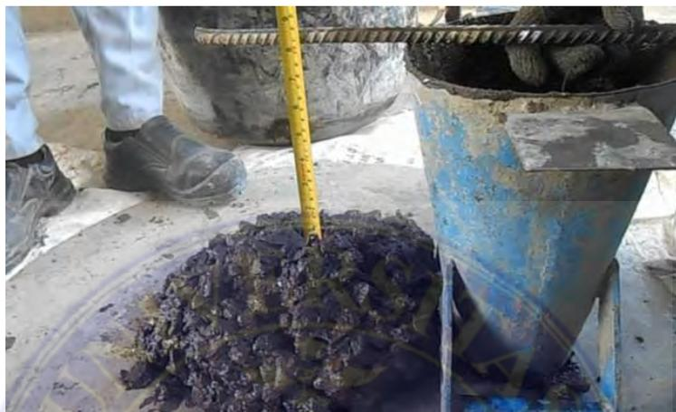
Gambar 9. Slump Test
