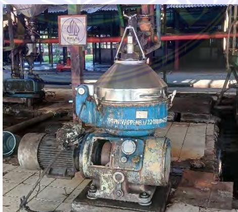
**Gambar 3. 44 Sludge Separator**
