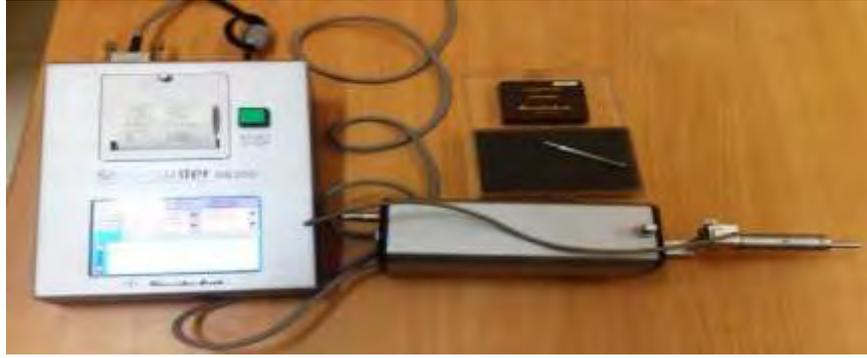
Gambar 2.14. *Surface Roughness Tester* Kosaka Japan
