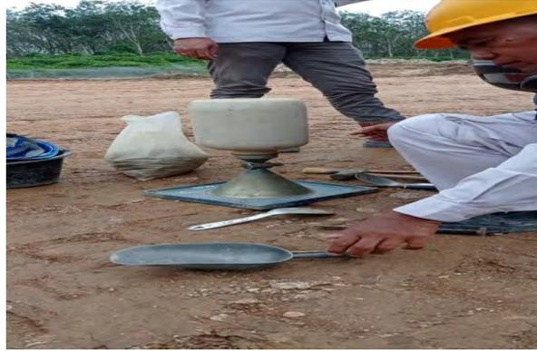
Gambar 4.2 *Test Sand Cone*
