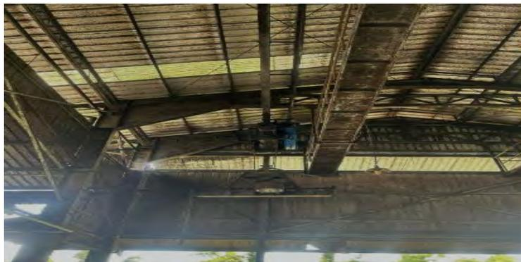
**Gambar 3. 13 *Hoisting Crane***
