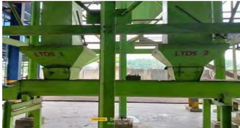
**Gambar 3.16. Ligh tenera dry separating (LTDS-2)**
