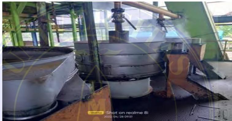
**Gambar 3.31. Oil Vibre Separator**
