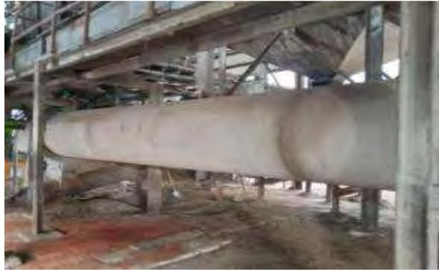
Gambar 3.45 Nut Polishing Drum
