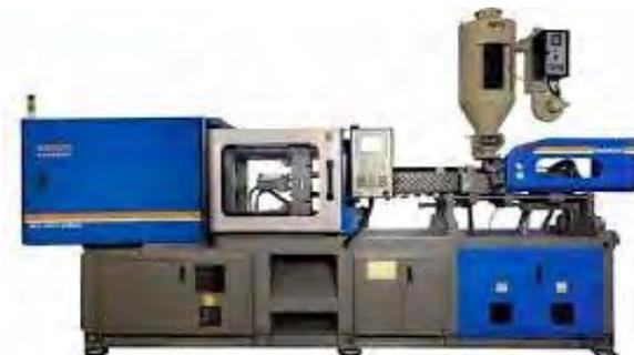
Gambar 2. 11. *Ijection molding* horizontal
