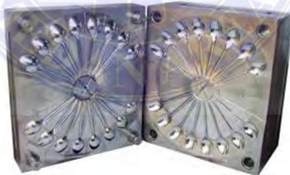
Gambar 2.12. Cetakan/ *Mold Injection Molding Vertical*
