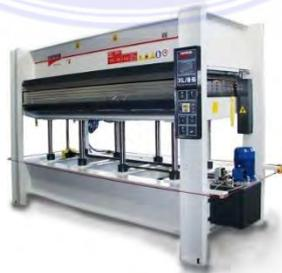
Gambar 2.5. *Multi-Daylight Hot Press*
