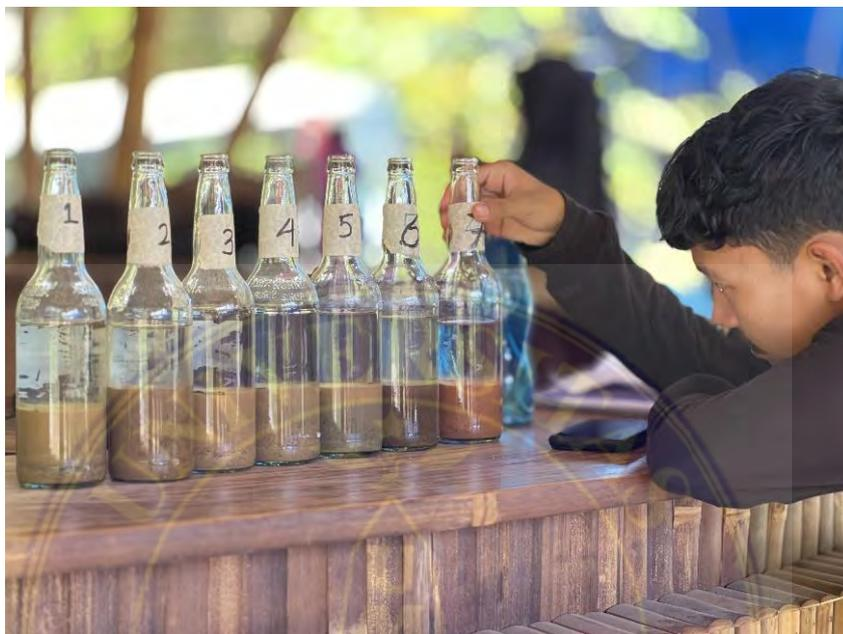
Gambar 5. 18 Sample Campuran Bahan Rammed Erath Wall
