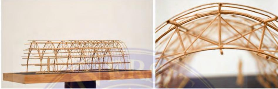
Gambar 2. 9 maket *Arched Truss Structures*
