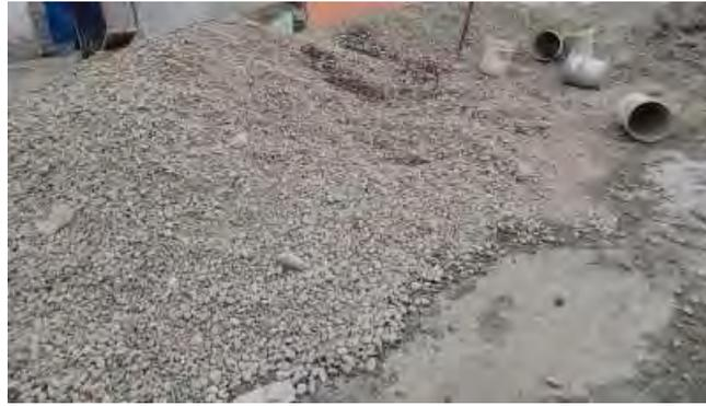
Gambar 23. Agregat (Batu Pecah )
