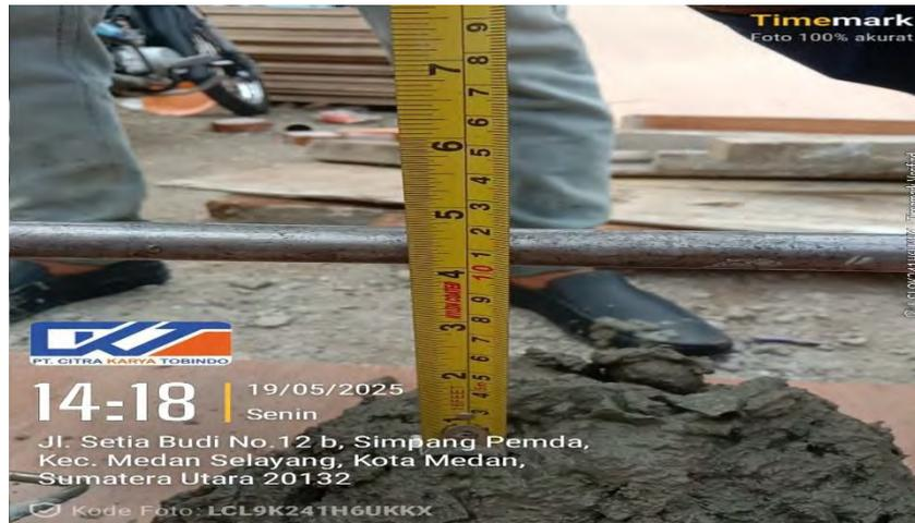
Slump Test Beton T-Beam
