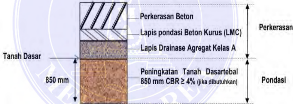
Gambar 2. Strukur Perkerasan Kaku (Manual desain perkerasan jalan No: 03/MN/B/2024)
