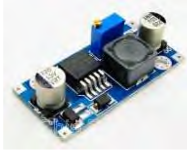
Gambar 2.5 Bentuk Fisik Adjustable Step-Down DC-DC (Sumber: https://www.voltaat.com/products/adjustable-buck-converter )
