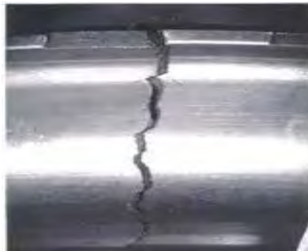
Gambar 2.4. Mekanis keausan Fretting Kelelahan.
