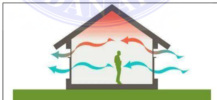
Gambar 2.3 Ilustrasi Cross Ventilation Sumber: www.voyerdesign.com
