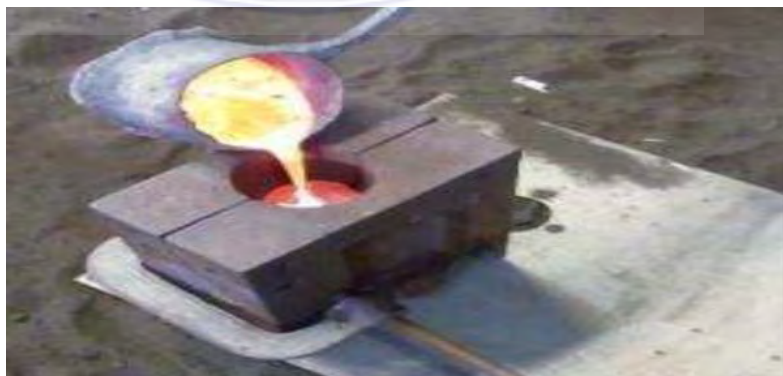
Gambar 2. 2 Proses Pengecoran Aluminium
