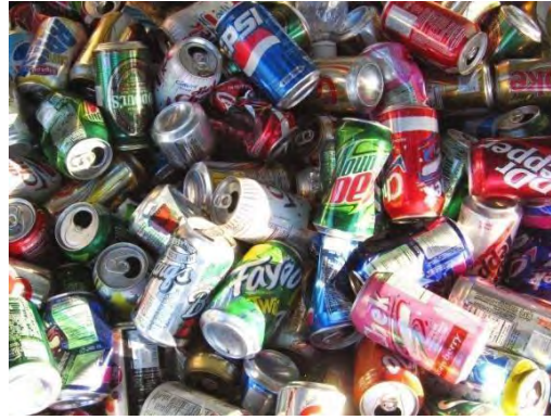
Gambar 2. 1 Material Kaleng Aluminium 3004
