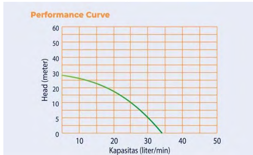
Gambar 3. 6 Grafik performa pompa Shimizu PS-116 BIT
