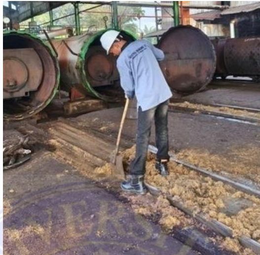
Gambar 3. 15 Pembersihan Rail Track
