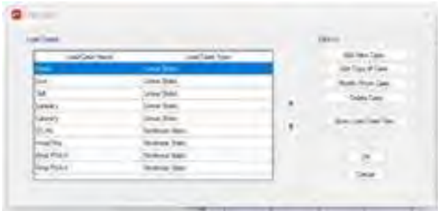
Gambar 40 Define Static Load Cases (ETABS V18, 2025)
