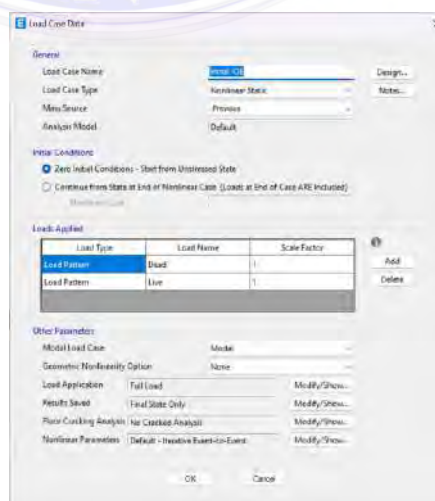
Gambar 34. Input Static Nonlinier Initial POA(ETABS V22, 2025)
