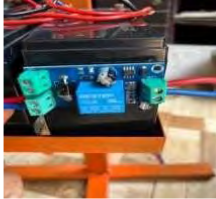
Gambar 3. 15 Modul UPS DC
