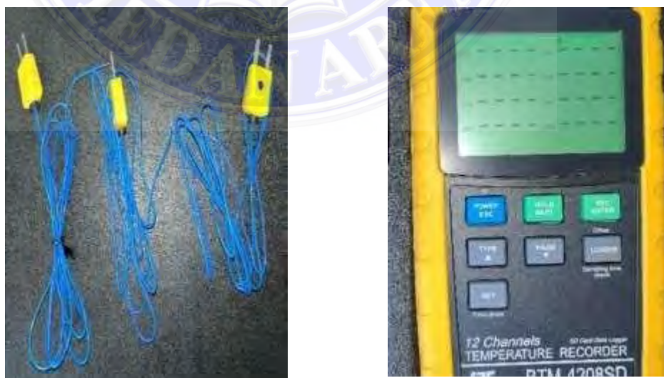
Gambar 3. 11 Termokopel data logger
