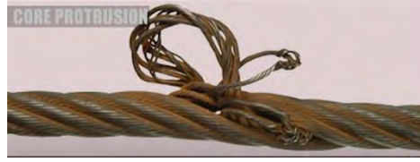
Gambar 3.16. kink, Bridcaging, dan core protrusion
