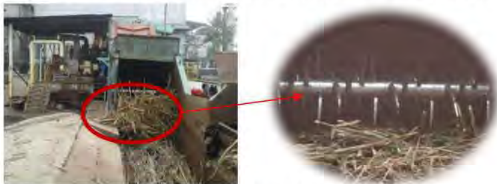
Gambar 3. 4 Cane Cutter I
