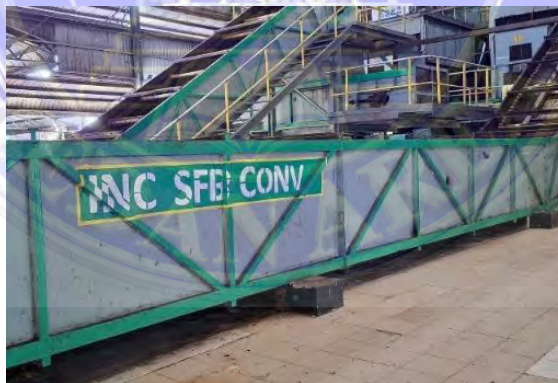
Gambar 3.19 INC SFB ( Inclined Sterilizer Fruit Bunch ) Scrapper
